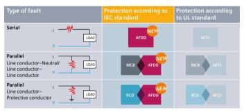
Figure 12: Fault types and protective devices suitable for fire protection
