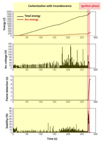
Figure 16: Development of the arc using the example 2 A / 230 V
