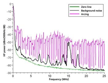
Figure 28: High-frequency noise: Background noise and arcs
