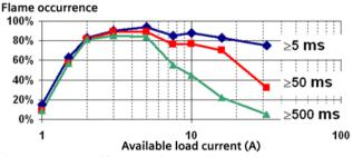
Figure 19: Outbreak of flames as a function of load current
