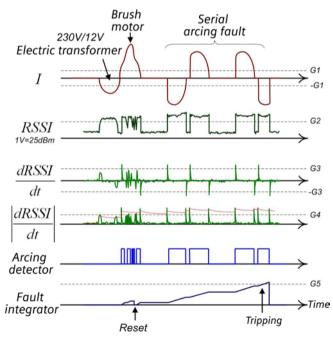
Figure 24: Signal processing for assessing serial arcing faults
