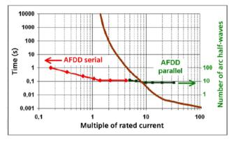
$\rightarrow$  n-times the rated current (AFD unit with I<sub>n</sub> = 16A) Figure 22: Protection by fuse
