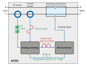
Figure 23: Basic design of the 5SM6 AFD unit
