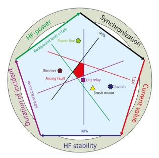
Figure 27: Factors for the detection of an arcing fault
