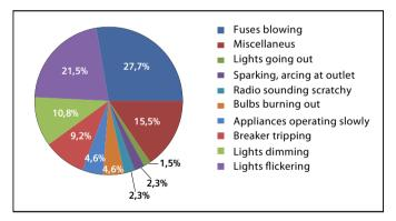
Figure 6: Observations made in the USA before the outbreak of fires caused by electricity
