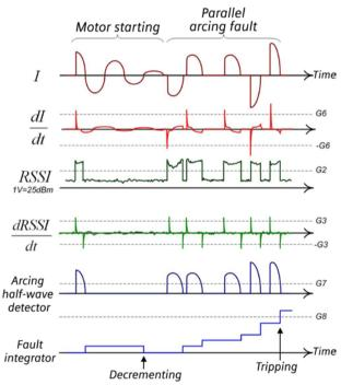
Figure 25: Signal processing for assessing parallel arcing faults
