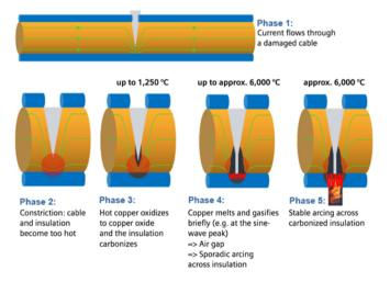
Figure 15: Outbreak of a fire due to serial arcs
