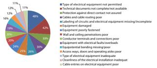
Figure 2: Statistics of defects in electrical systems (2007)
