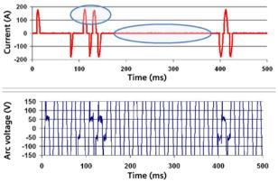
Figure 20: Current and voltage curve for a parallel arcing fault
