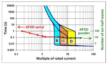
$\rightarrow$  n-times the rated current (AFD unit with I<sub>n</sub> = 16A) Figure 21: Protection by MCB
