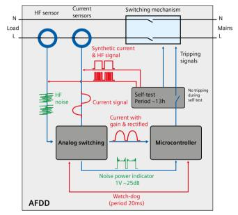
Figure 31: Diagram of the internal self-test function
