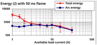
Figure 18: Energy of the significant flame as a function of load current
