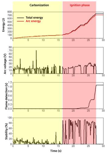
Figure 17: Development of the arc using the example 5 A / 230 V
