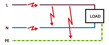
Figure 11: Types of arcing fault
