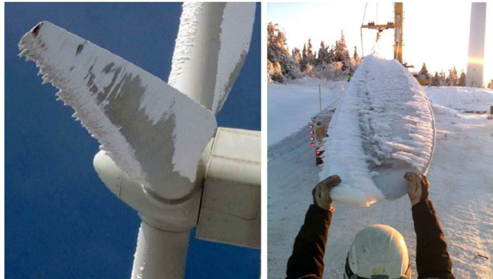
Figure 13. Ice on wind turbine blades [69,76].
