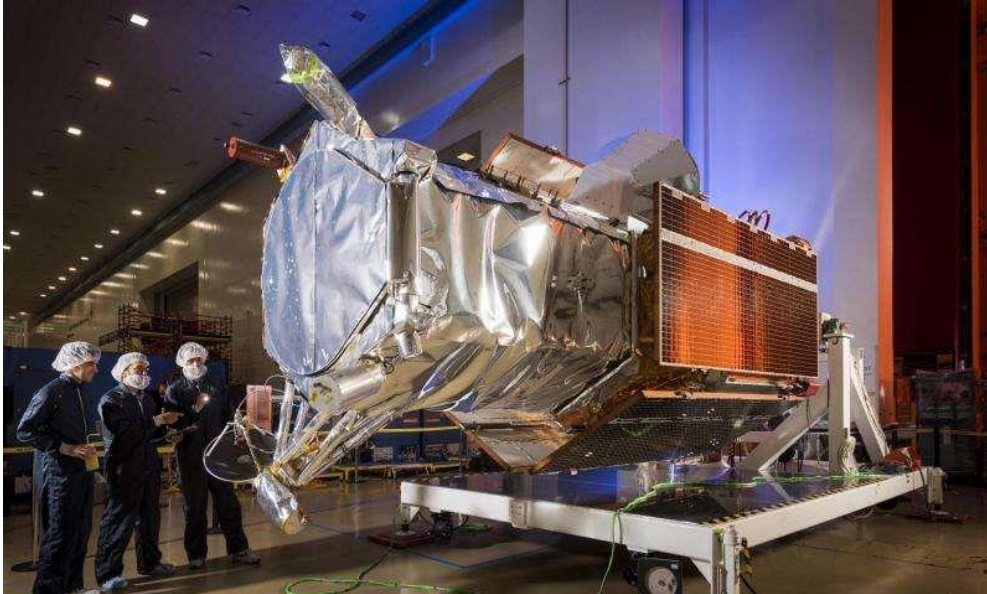
Big Space: DigitalGlobe's state-of-the-art Worldview-4, capable of 30cm resolution imagery, undergoes prelaunch checks, prior to launch in 2016 (Image -Lockheed Martin)
