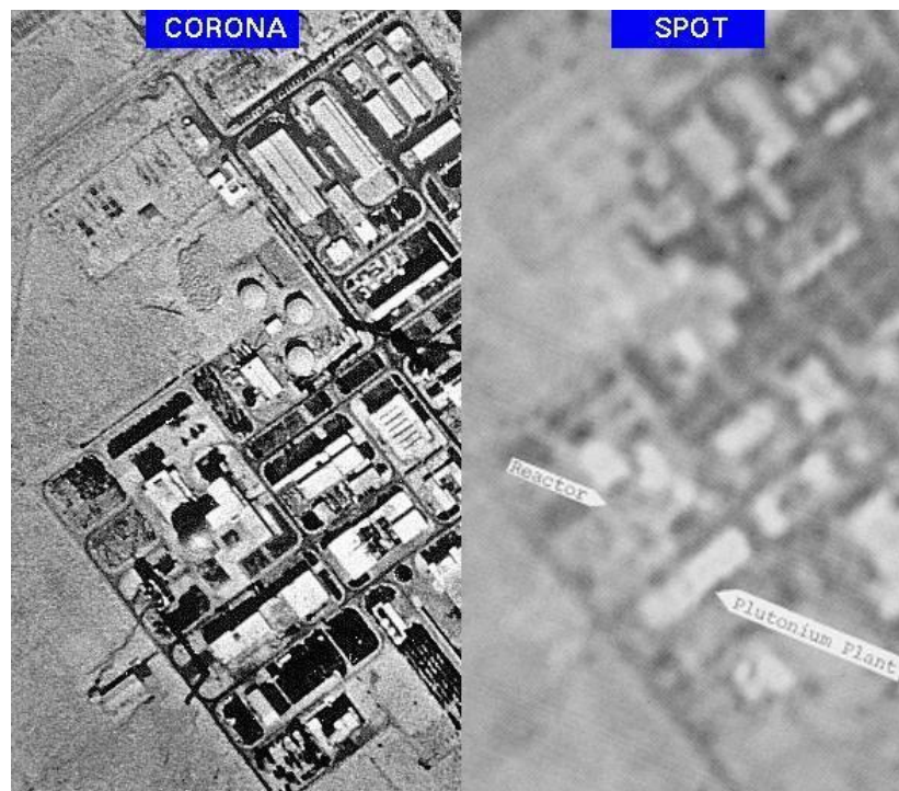
Israel's Dimona nuclear weapons production facility. Side by side comparison of Corona US spy satellite image from 1971, declassified in 1996, and the much lower resolution image by French commercial satellite SPOT, recorded in 1996 (Images – Federation of American Scientists/US Government/SPOT)
